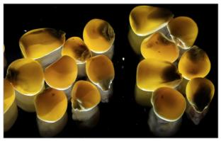
Visualization of vitreousness and cracks in corn
