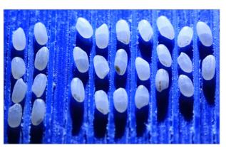
Visualization of internal cracks on milled rice
